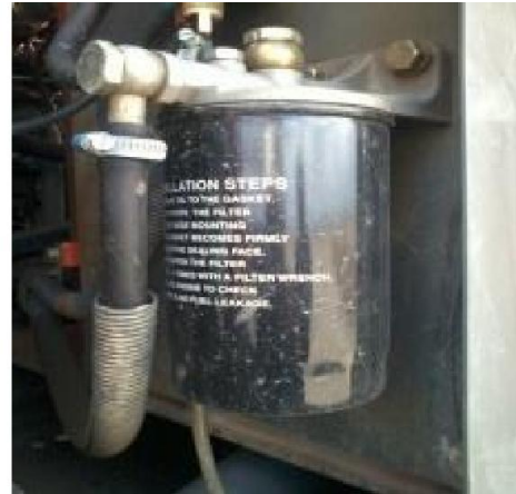
Gambar 4.8 Primary oil filter
