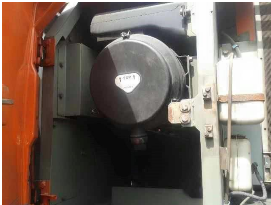
Gambar 4.21 Filter udara
