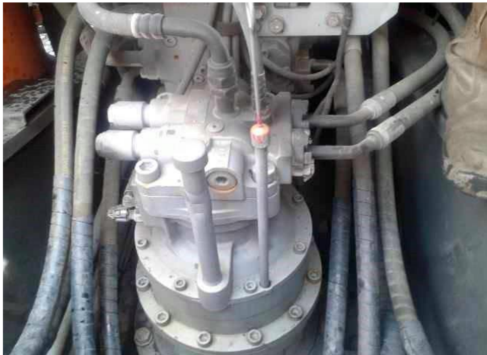
Gambar 4.17 Swing reduction gear
