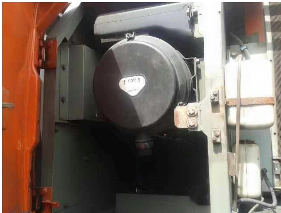
Gambar 4.21 Filter udara
