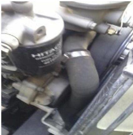
Gambar 4.9 Secondary oil filter
