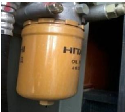
Gambar 4.11 Hydraulic pilot filter
