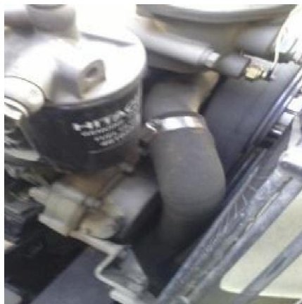
Gambar 4.9 Secondary oil filter
