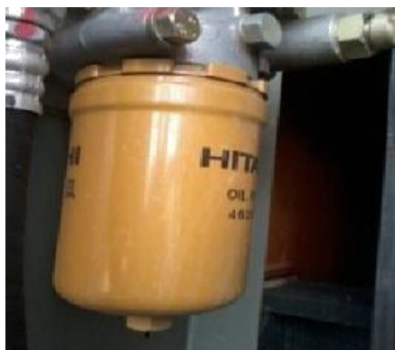
Gambar 4.11 Hydraulic pilot filter
