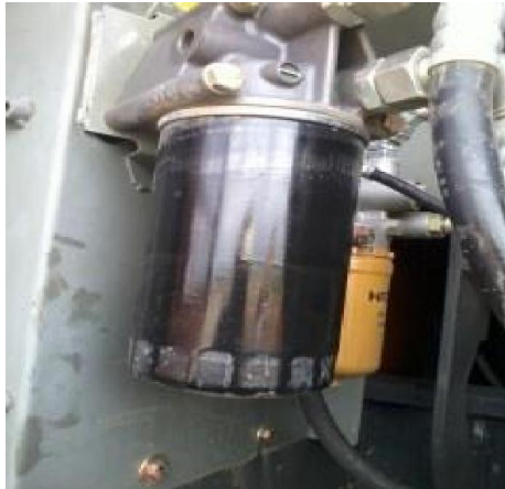
Gambar 4.7 Engine oil filter
