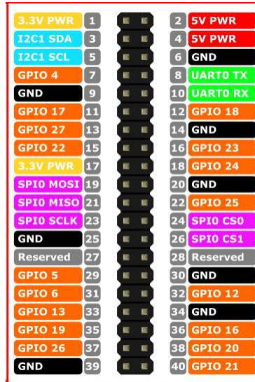
Gambar 2.13 Pin GPIO Raspberry Pi 3B (raspberrypi.org, 2016)
