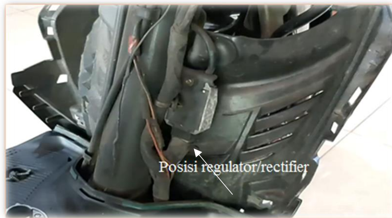
Gambar 3.7 Posisi regulator/rectifier Soul GT 115
