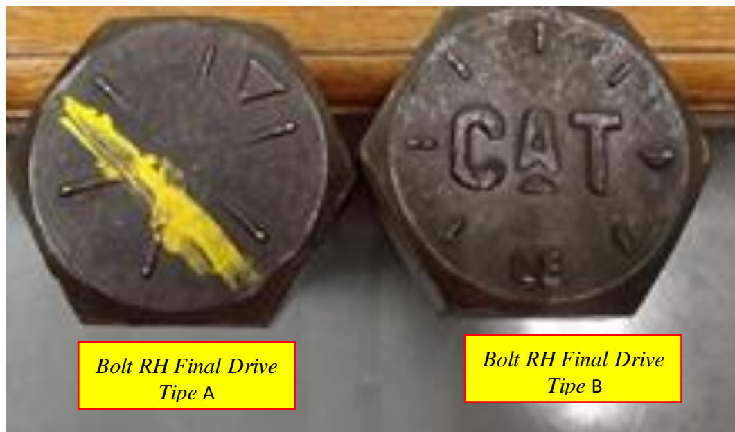
Gambar 4.12 Tipe baut final drive
