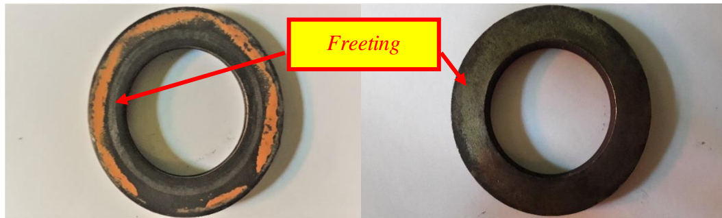
Gambar 4.15 Ring baut final drive fretting
