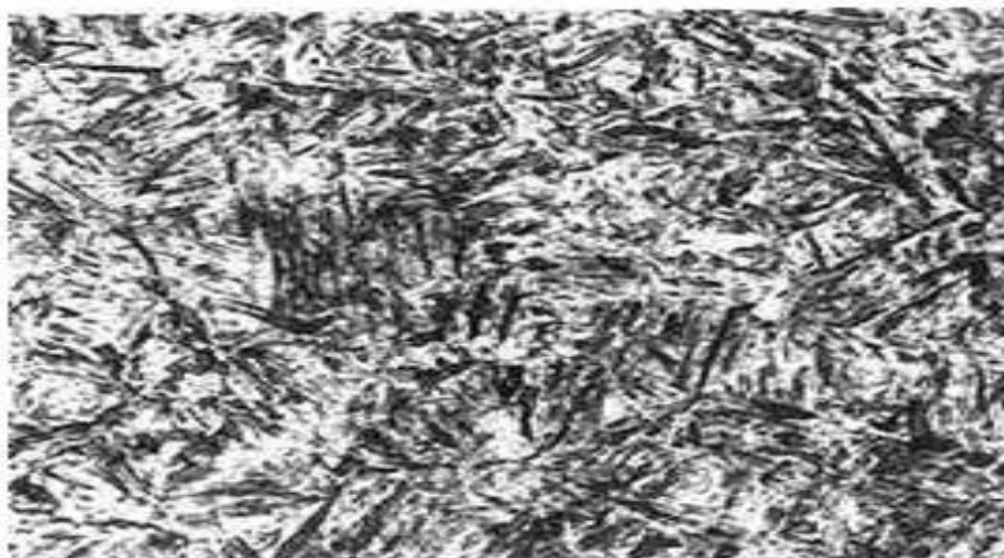
Gambar 2.14 Struktur martensite (Mettallurgy, 2018)
