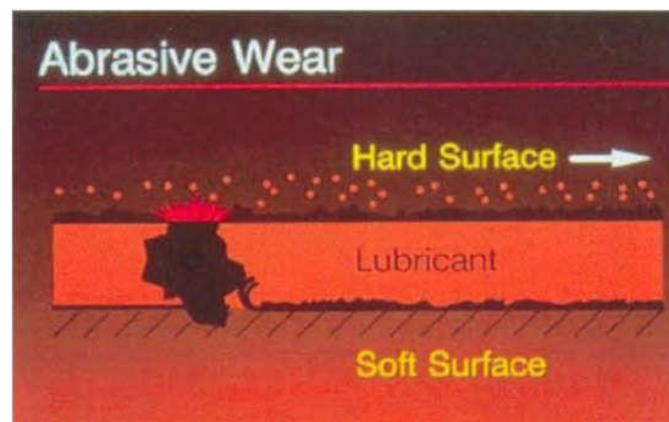
Gambar 2.23 Abrasive wear (Trakindo, 2014)
