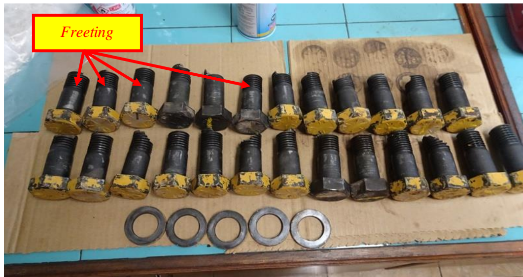
Gambar 4.11 Baut final drive patah
