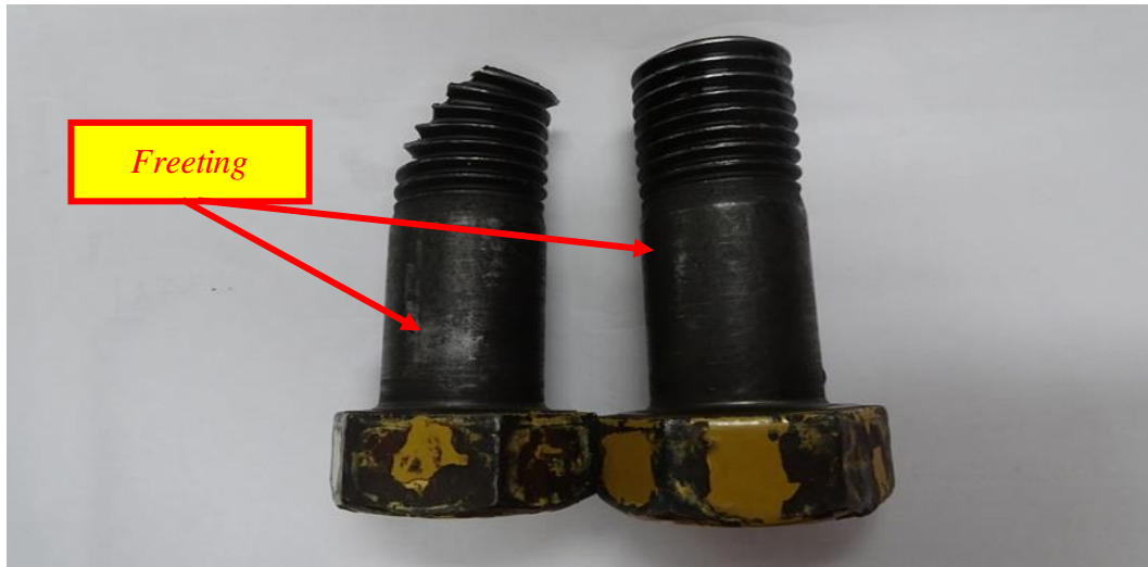
Gambar 4.13 Baut final drive fretting on the shank
