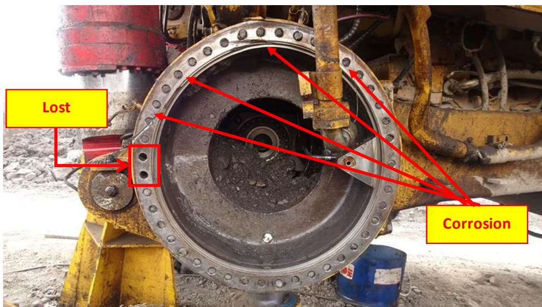
Gambar 4.6 Hoist differential
