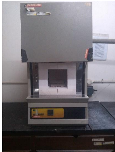
Box furnace (CarboliteRHF 16/3)
