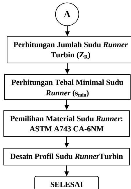
Gambar 3.2. Flowchart Perancangan Runner (Roda Gerak) Turbin
