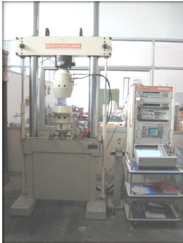
Gambar 3.4 Alat Uji Tarik Universal Servopulser
