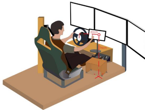
Figure 4.10 High Installation 3D
