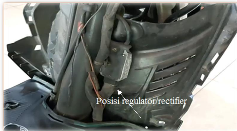
Gambar 3.7 Posisi regulator/ rectifier Soul GT 115
