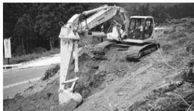
Gambar 2. 8 Two Piece Boom
